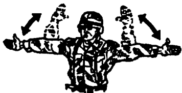
HERRINGBONE. Extend the arms parallel to ground. Bend the arms until the forearms are perpendicular. Repeat.
